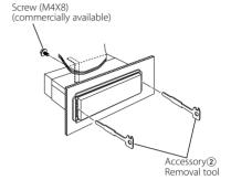
**4** Lower the removal tool toward the bottom, and pull out the unit halfway while pressing towards the inside.
